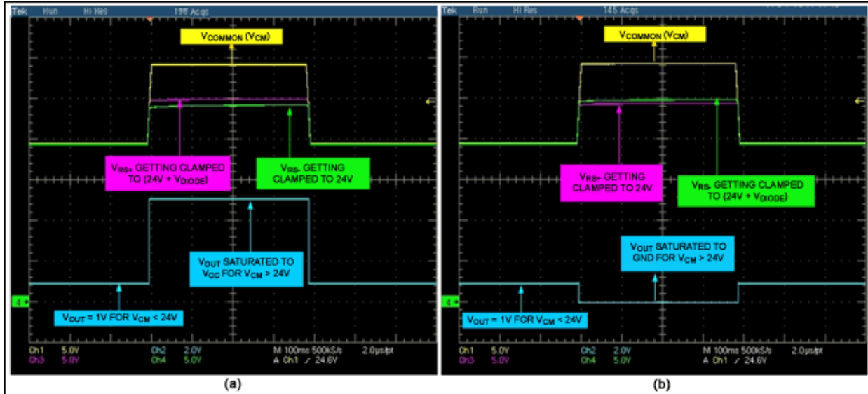
Figure 3. Operation of the Figure 1 circuit with D1 in series with Z1 (a), and D1 in series with Z2 (b).
