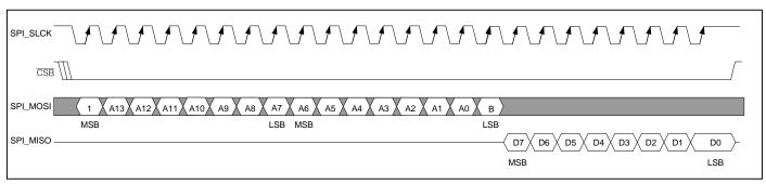
Figure 9-5. SPI Serial Port Access for Write Mode, SPI\_CPOL = 0, SPI\_CPHA = 0
