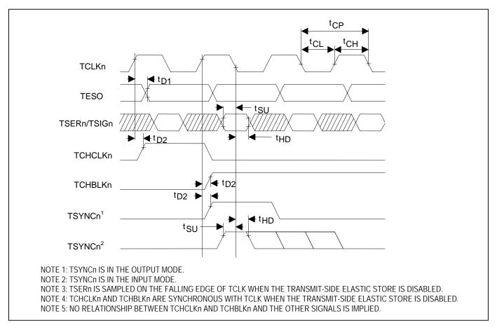
Figure 13-10. Transmit Formatter Timing—Elastic Store Enabled
