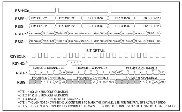
Figure 11-23. E1 Receive-Side RCHCLKn Gapped Mode During Channel 1
