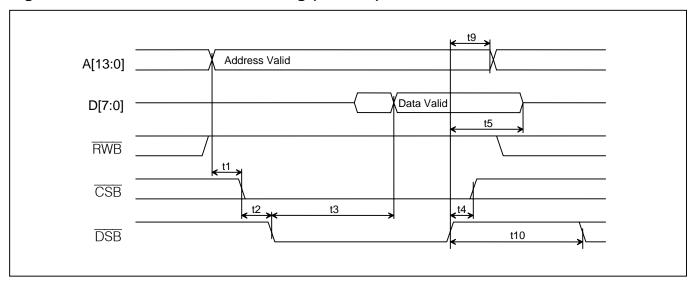
Figure 13-5 Motorola Bus Write Timing (BTS = 1)
