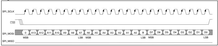
Figure 9-6. SPI Serial Port Access for Write Mode, SPI\_CPOL = 1, SPI\_CPHA = 0
