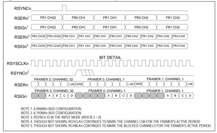
Figure 11-22. E1 Receive-Side Interleave Bus Operation—FRAME Mode
