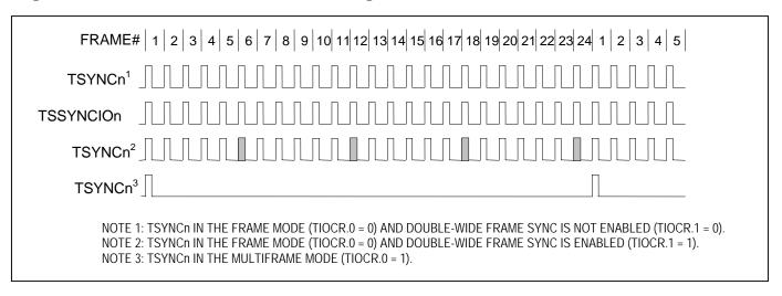
Figure 11-11. T1 Transmit-Side Boundary Timing (Elastic Store Disabled)
