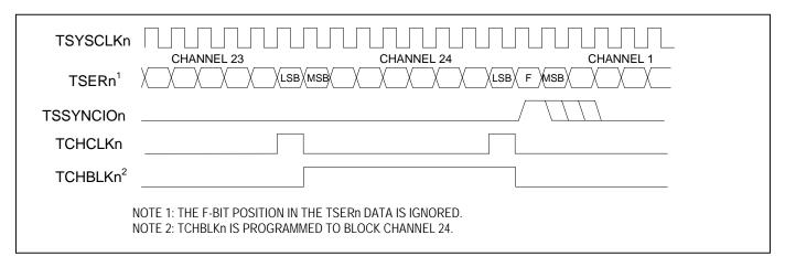
Figure 11-27. E1 Transmit-Side 2.048MHz Boundary Timing (Elastic Store Enabled)
