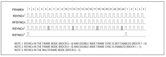
Figure 11-3. T1 Receive-Side Boundary Timing (Elastic Store Disabled)
