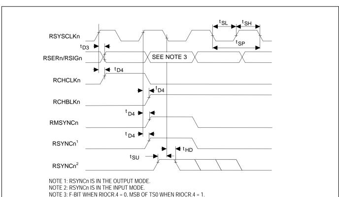
Figure 13-7. Receive-Side Timing—Elastic Store Enabled (T1 Mode)
