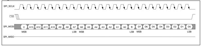
Figure 9-8. SPI Serial Port Access for Write Mode, SPI\_CPOL = 1, SPI\_CPHA = 1
