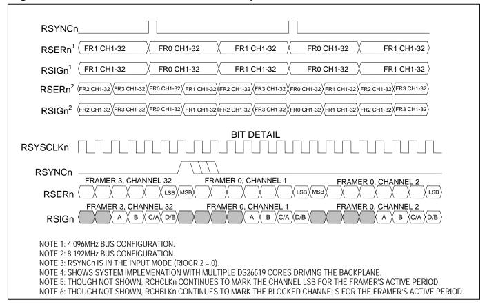
Figure 11-8. T1 Receive-Side RCHCLKn Gapped Mode During F-Bit
