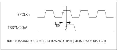
Figure 13-12. Transmit Formatt Timing—Line Side
