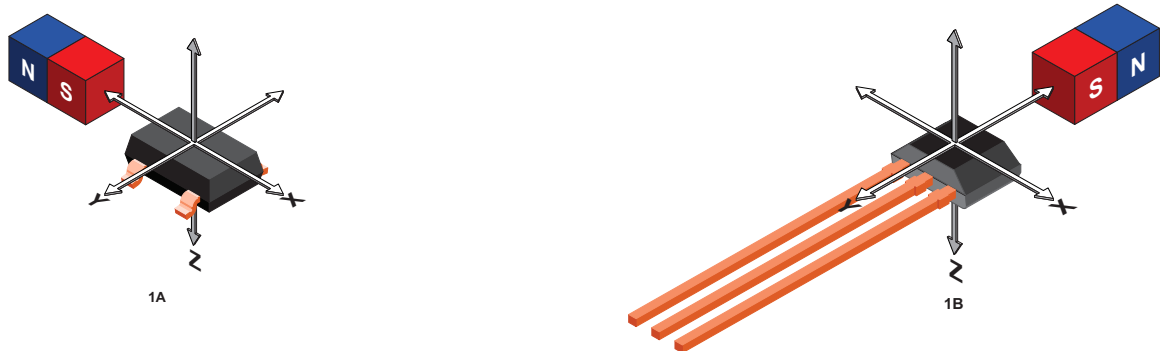
Figure 1: Magnet Orientation for Switching Output On for LH package (Panel 1A) and UA Package (Panel 1B)
