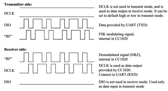
Figure 5-8. Transparent Asynchronous UART Mode (SEP\_DI\_DO = 1)
