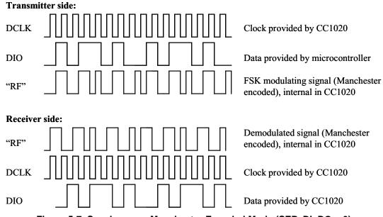
Figure 5-7. Synchronous Manchester Encoded Mode (SEP\_DI\_DO = 0)
