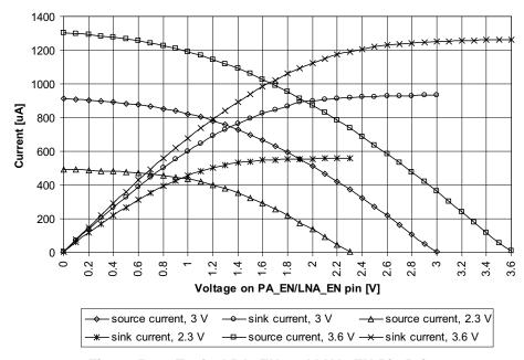
Figure 5-32. Typical PA\_EN and LNA\_EN Pin Drive
