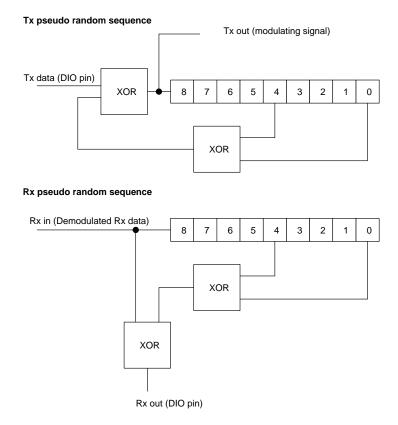
Figure 5-31. PN9 Pseudo-random Sequence Generator in TX and RX Mode
