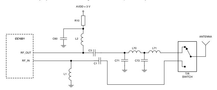
Figure 5-22. Input and Output Matching Network
