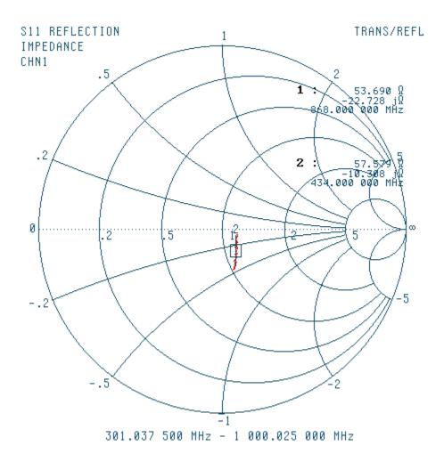
Figure 5-23. Typical LNA Input Impedance, 200 to 1000 MHz
