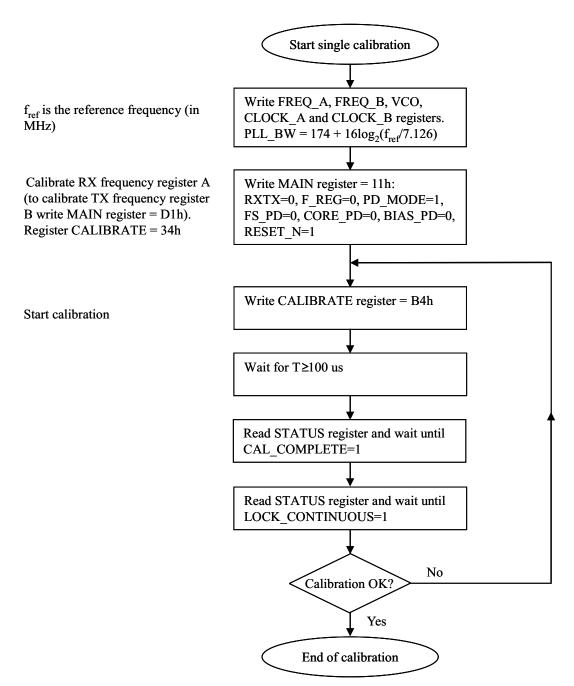
Figure 5-26. Single Calibration Algorithm for RX and TX
