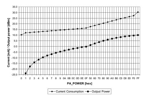
Figure 5-20. Typical Output Power and Current Consumption, 433 MHz
