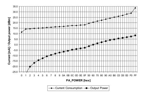
Figure 5-21. Typical Output Power and Current Consumption, 433 MHz
