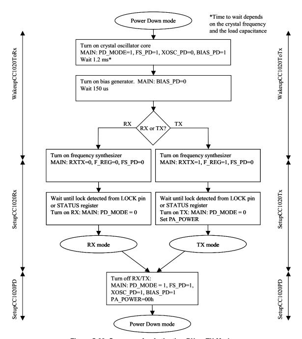
Figure 5-28. Sequence for Activating RX or TX Mode
