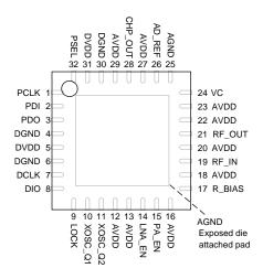
Figure 3-1. Package 7-mm × 7-mm VQFNP (Top View)
