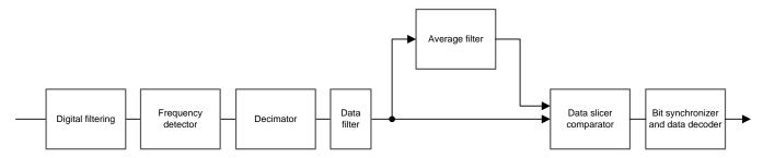
Figure 5-10. Demodulator Block Diagram
