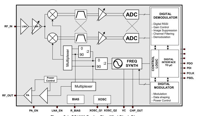
Figure 5-1. CC1020 Device Simplified Block Diagram
