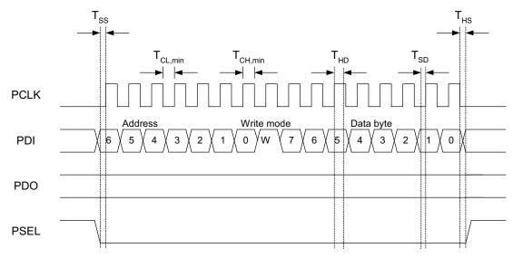
Figure 5-4. Configuration Registers Write Operation
