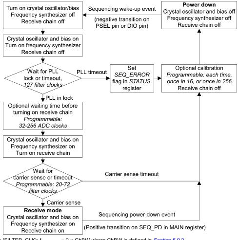
(1) Filter clock (FILTER\_CLK): f<sub>filter clock</sub> = 2 x ChBW where ChBW is defined in Section 5.9.2.
