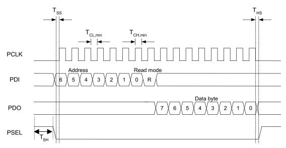
Figure 5-5. Configuration Registers Read Operation
