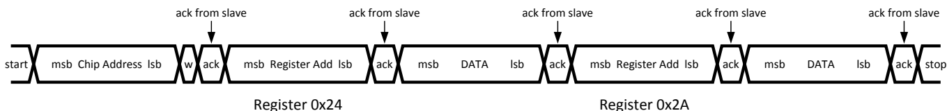
Figure 23. Multi-Byte I 2 C Command
