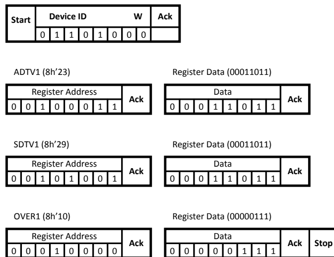
Figure 25. SOD Multi-Byte Random Register Transfer
