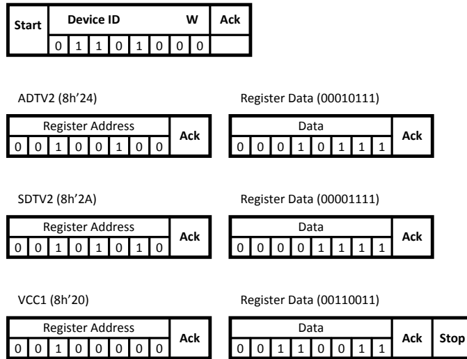
Figure 26. Master and Slave Data Exchange
