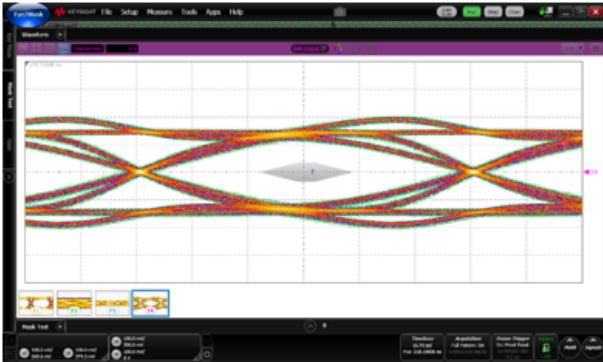
Figure 7. USB3.1 Gen 2 10.0 Gbps eye diagram without ECMF4-20A42N10 (test conditions: type C connector, reference cable equalizer with A_{DC} = 6 dB and DFE)
